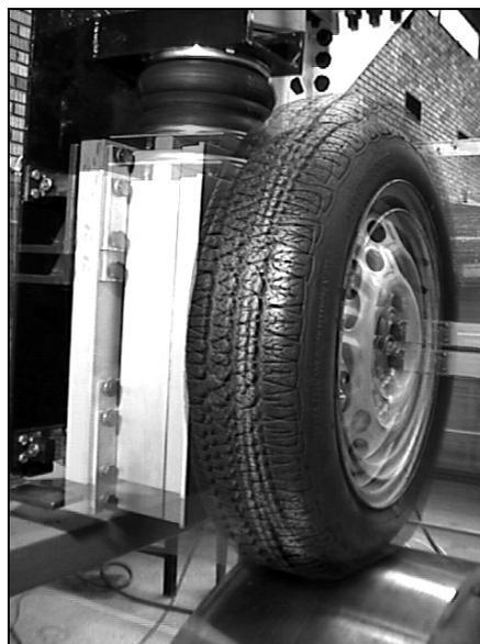
Figure 3.2 The Vertical Tire Motion under Load
