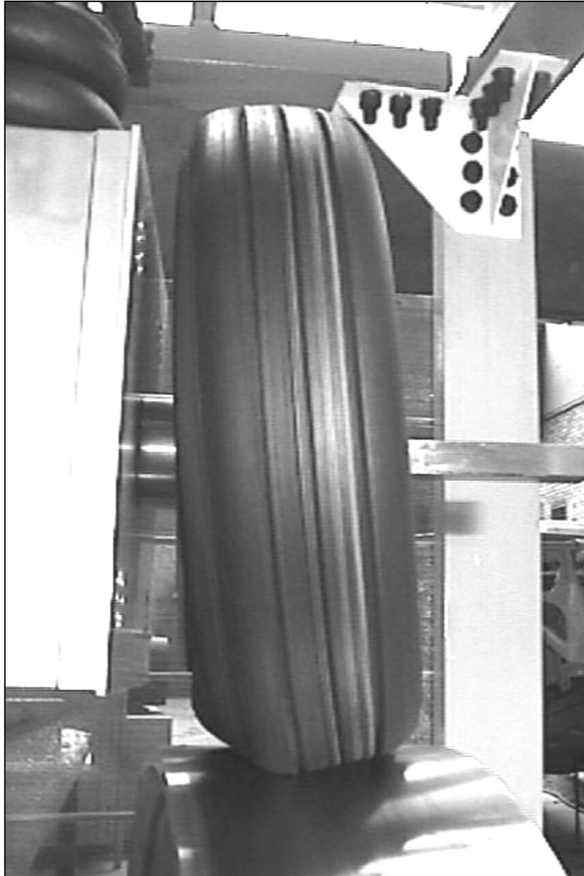
Figure 7.1 Deformed Photograph of 155R13 Tire
