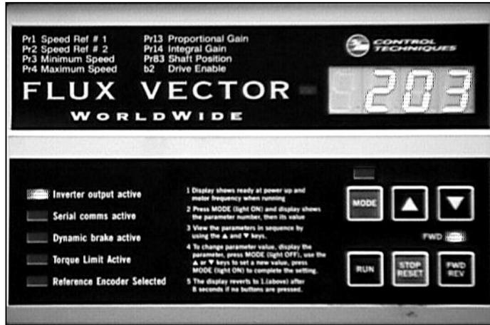
Figure 3.6 The Control Pod of Speed Controller
